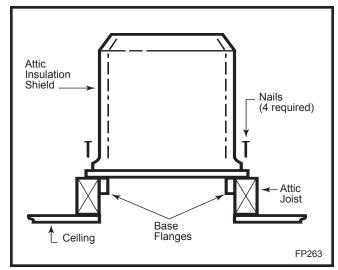
Fig. 19 Attic shield installlation (Canadian requirement).
